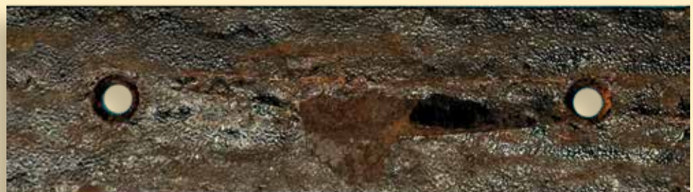
Close up of Deliberate Scratch shows excessive rust, dramatic rust migration, and advanced detachment of the surface coating
